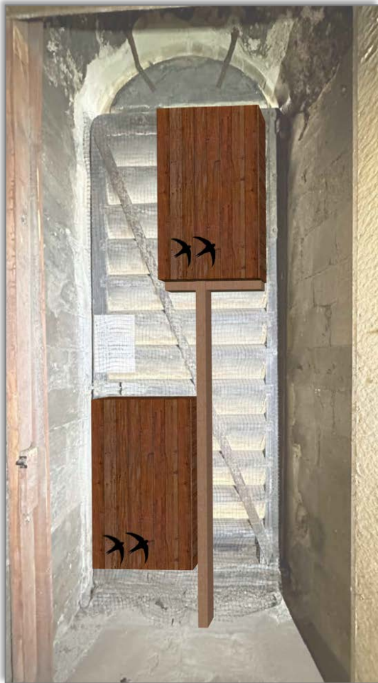
Fig. 2: Proposed design of nestboxes and location in relation to existing features.
